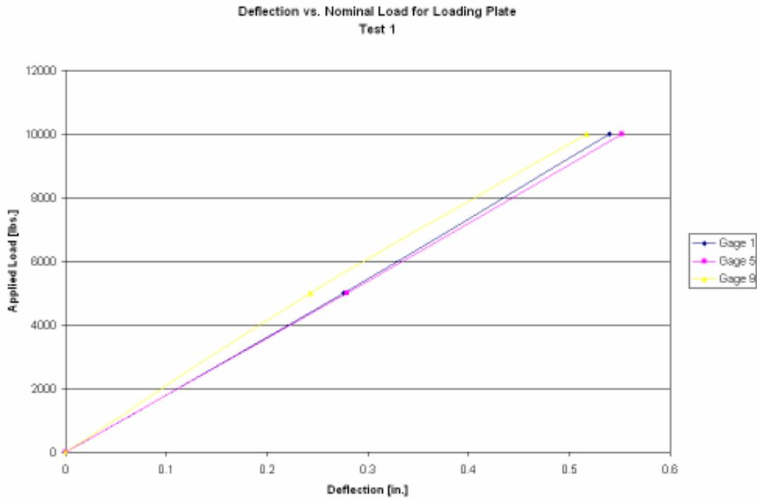
**Figure 5:** Vertical Deflections and Nominal Loads Measured at the Loading Plate for Test 1
