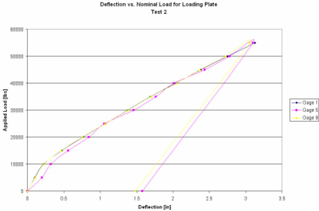
**Figure 7:** Vertical Deflections and Nominal Loads Measured at the Loading Plate for Test 2
