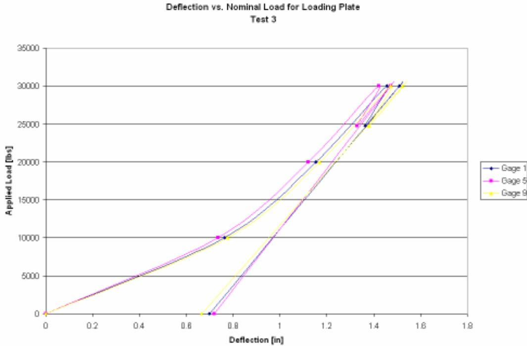
**Figure 9:** Vertical Deflections & Nominal Loads Measured at the Loading Plate for Test 3
