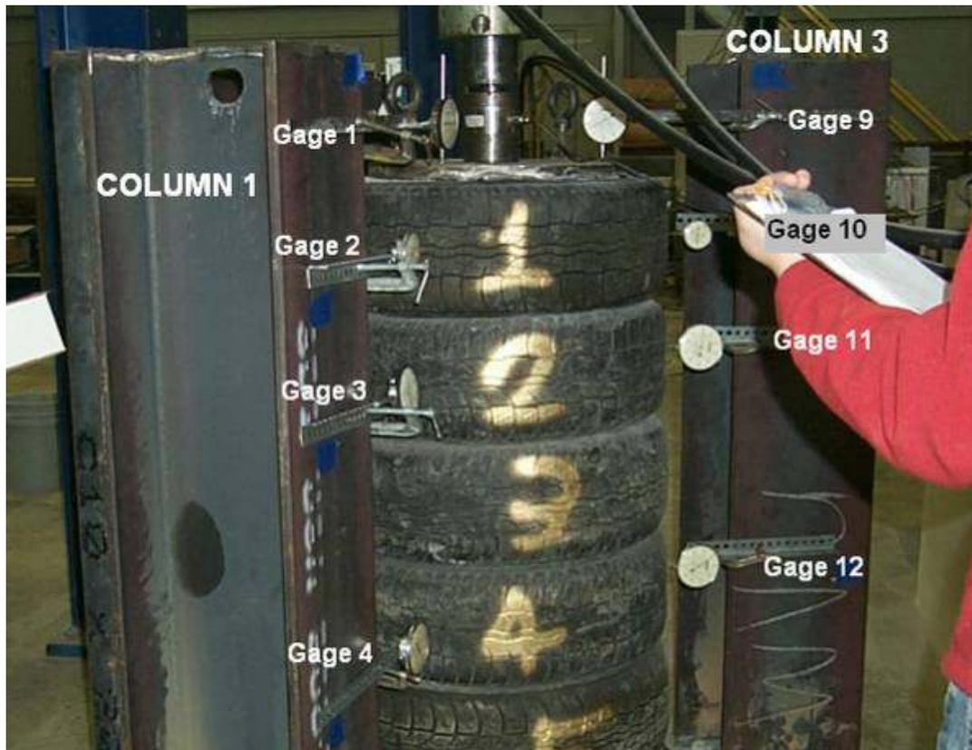
**Figure 3:** Attachment System Used for Holding Dial Gages in Place and Numbering System for Steel H Columns and Dial Gages (Steel H Column 2 Not Visible)
