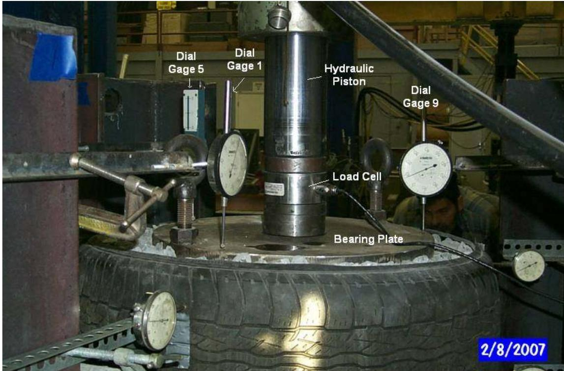
**Figure 2:** View of Testing Equipment and Instrumentation at Top of Tire Column
