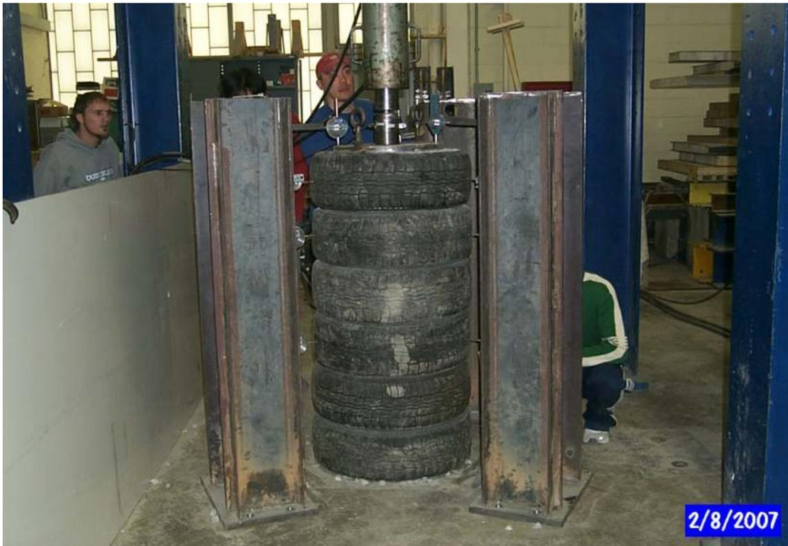
**Figure 1:** Tire Tread Cylinder CAC Column with Instrumentation
