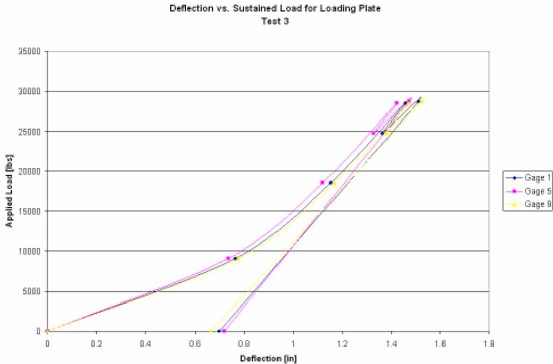
**Figure 10:** Vertical Deflections and Sustained Loads Measured at the Loading Plate for Test 3
