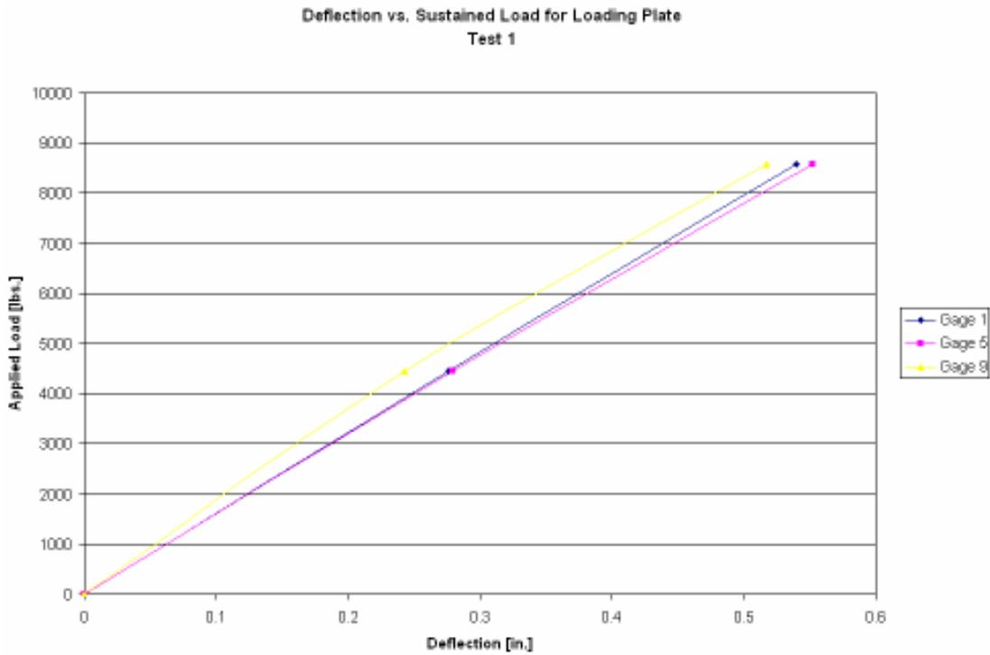
**Figure 6:** Vertical Deflections and Sustained Loads Measured at the Loading Plate for Test 1
