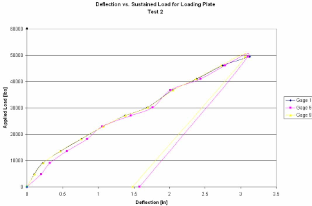
**Figure 8:** Vertical Deflections and Sustained Loads Measured at the Loading Plate for Test 2
