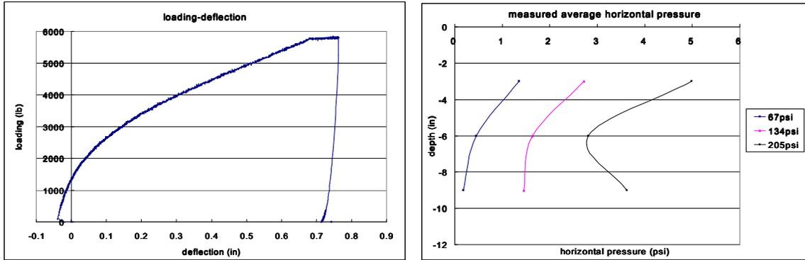
12" tube 12" plate 3/4 inch crusher-run (23,000lb max) (HS 20 Wheel 16,000lbs / 100psi)
