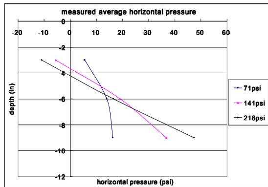
12" tube / 18" plate sand (50,000lb max) (HS 20 Wheel 16,000lbs / 100psi)
