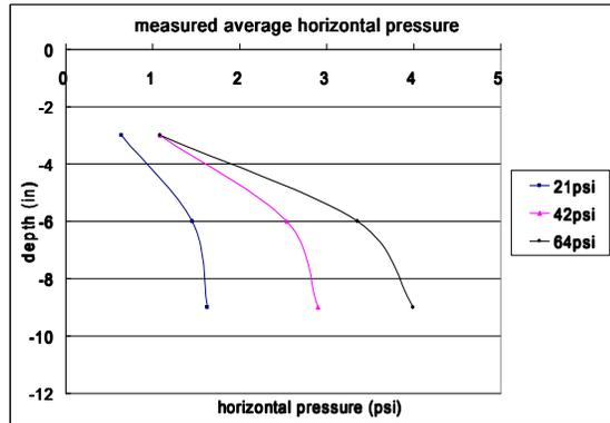
12" tube / 12" plate sand (23,000lb max) (HS 20 Wheel 16,000lbs / 100psi)
