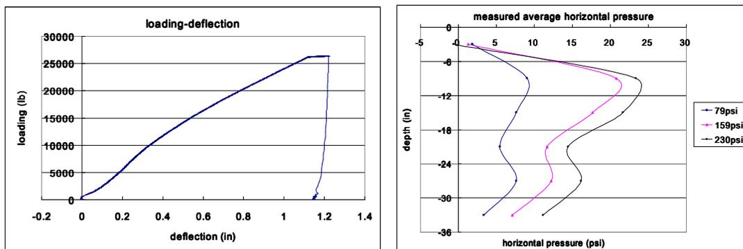
36" tube 18" plate 3/4 inch crusher-run (50,000lb max) (HS 20 Wheel 16,000lbs / 100psi)
